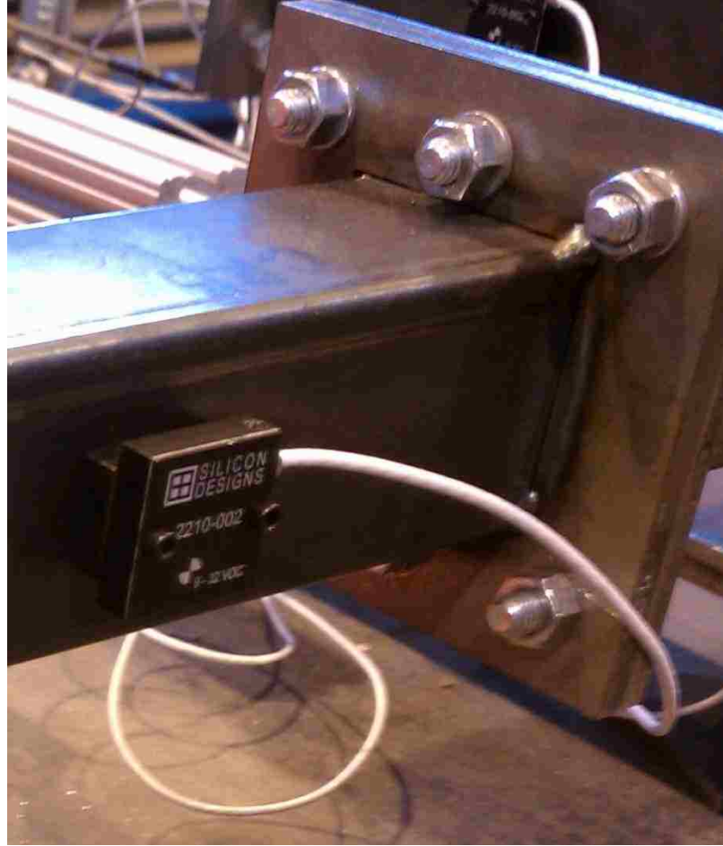
Figure 4.21. Silicon Designs 2210-002 wired accelerometer mounted on the frame
