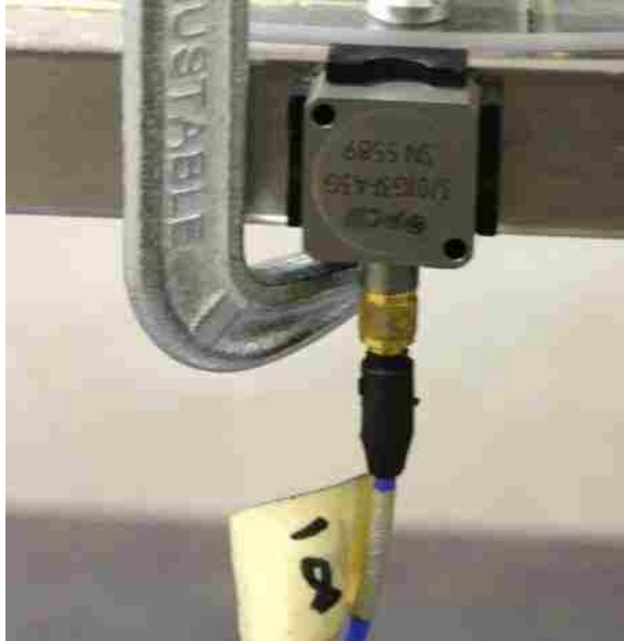
Figure 3.8. PCB 3701G3FA3G accelerometer mounted on beam at node 8
