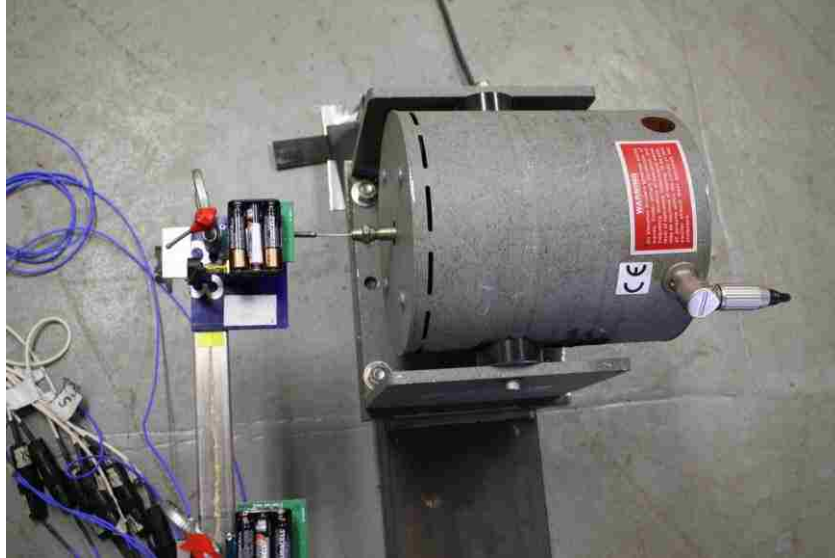
Figure 3.6. MODAL 50A by MB Dynamics actuator attached to free end of beam
